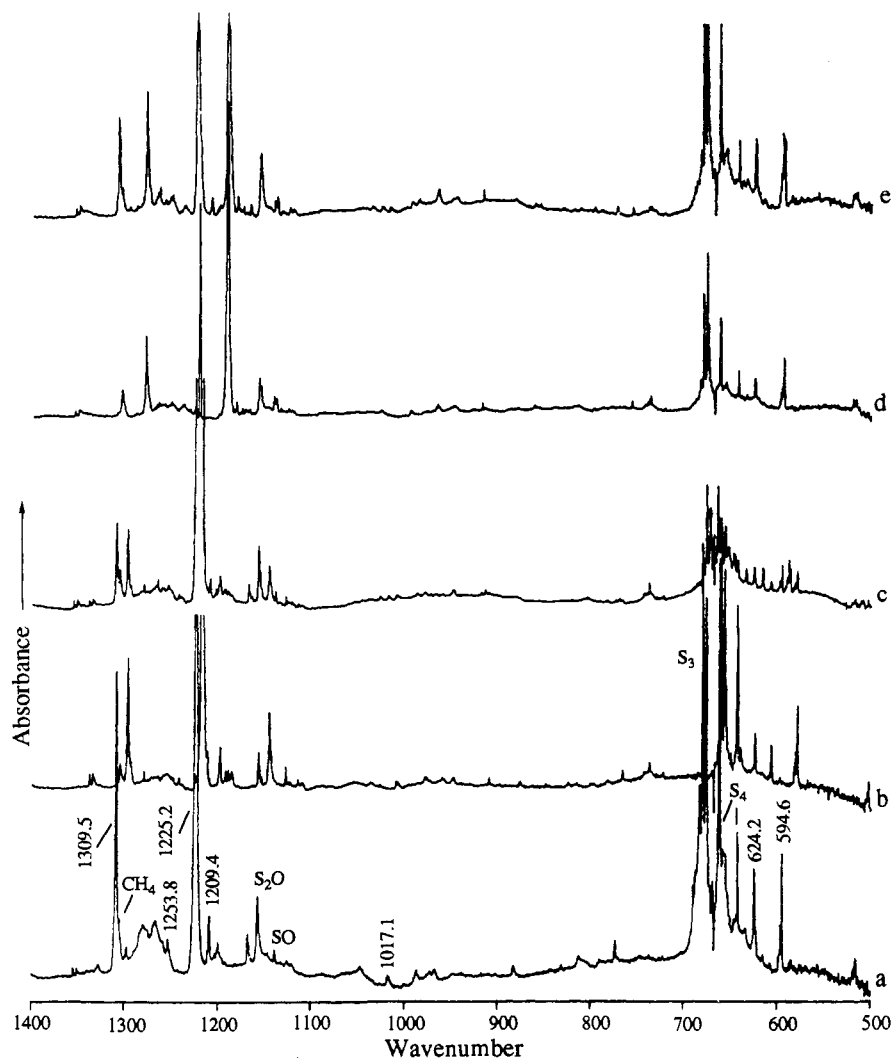
Figure 4. Infrared spectra in the 1400–500- \text{cm}^{-1} region for the discharged sulfur vapor/nitrogen/argon stream deposited on a CsI window at 12 \pm 1 K: (a) natural isotopic sulfur, (b) 98% ^{34}\text{S} -enriched sulfur, (c) 50% ^{34}\text{S} -enriched sulfur, (d) 99% ^{15}\text{N} -enriched nitrogen, and (e) 50% ^{15}\text{N}_2 and 50% ^{14}\text{N}_2 .
